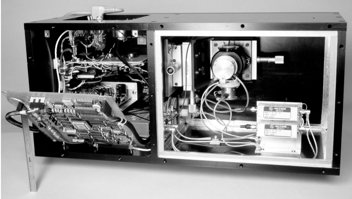
Figure 4.2. The Harvard targeted search photometer, with covers removed. Light enters from the rear of the righthand compartment, focused onto a 30 arcsec aperture, then passes through a beamsplitter onto the pair of HAPDs on their 3-axis stage. The detectors run at a gain of \sim 4 \times 10^4 , producing \sim 50 \mu\text{V} negative pulses into 50 \Omega , which are amplified and sent to the electronics in the lefthand compartment. The latter perform coincidence, 4-level ADC, timing, logging, hot-event veto, and communication with the host Linux PC. The photometer measures 25 \times 25 \times 60 cm, and weighs 30 kg.
